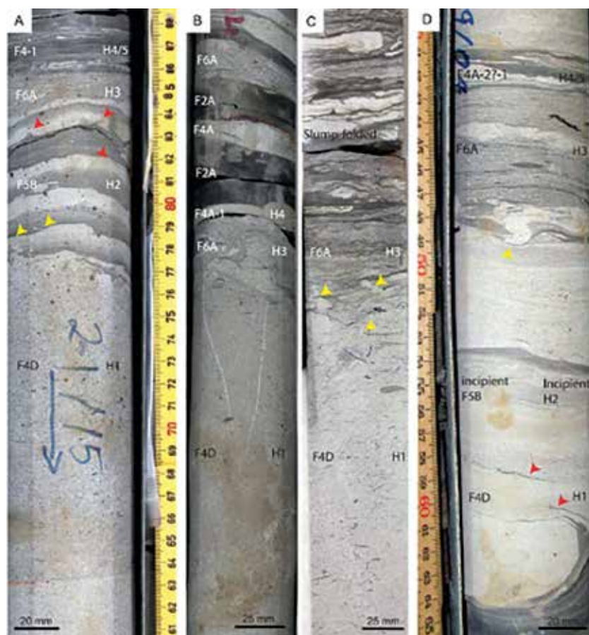
Figure 7. Core segments from syn rift sediments of well ENRECA-3 [3, 7].
